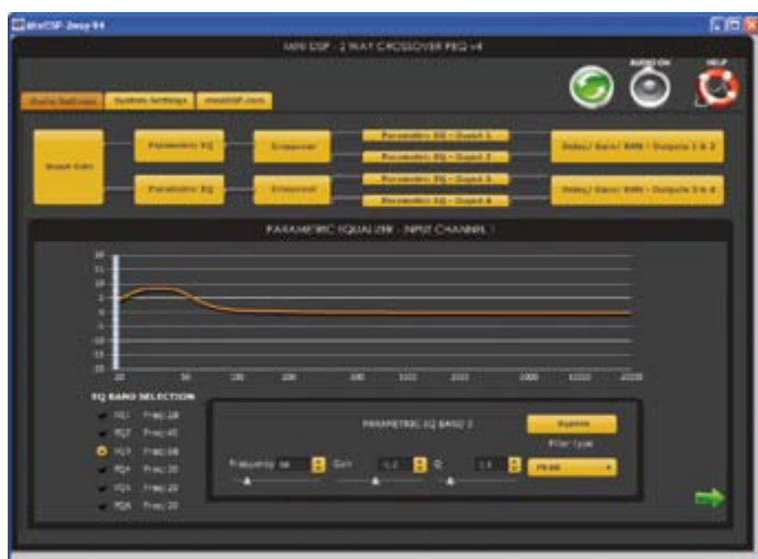
Figure 6. Every parametric equaliser of the two-way plug-in allows a maximum of six corrections (frequency, value, Q factor). Here a simple bass-boost has been realised.
