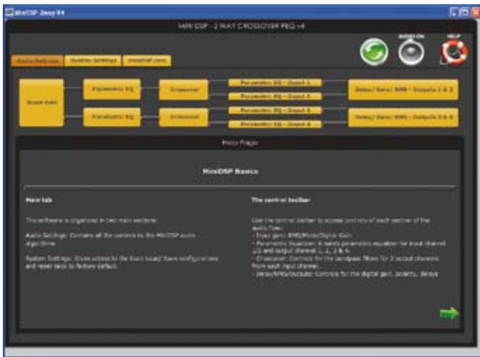
Figure 4. The design of the software. From this overview you can select each function block.
