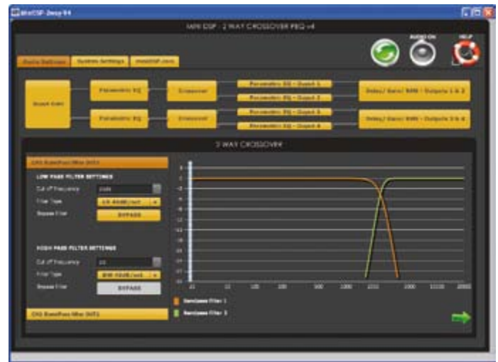
Figure 5. Here we can see the part for the crossover filter. You can select the crossover frequency, type of filter and slope. At the same time you can choose a band-pass filter.
